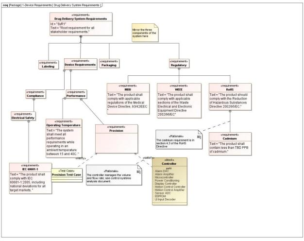
Fig. 3, Drug delivery device system requirements diagram
