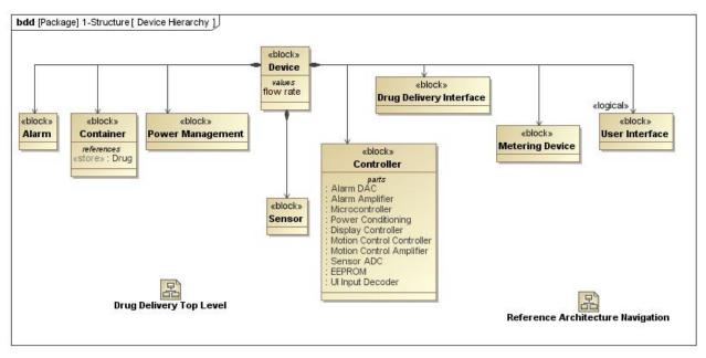
Fig. 4, Device hierarchy representing medical device sub-systems
